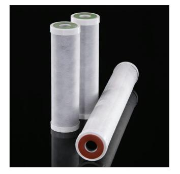
CARBOFLOW MX cartridges are offered in both high efficiency and general grades. They consist of bituminous coal sourced carbon, extruded together with an FDA listed thermoplastic binder, to produce an extremely porous yet rigid structure.
